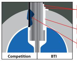
PTFE disc and stem encapsulation not only protects the disc but also extends up the stem, top and bottom. This extension along with a PTFE o-ring creates a leak proof seal against contamination.
