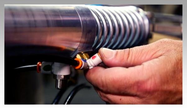
3. Push the Push/Pull valve IN and verify air comes out of the RED air line once the top casting is under all 5 wire forms
