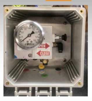
1. Verify the Push/Pull valve is pulled OUT and lid is in the open position
