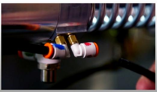
2. Remove the **RED** air line from elbow fitting on the air cylinder, this will keep the air bag from inflating
