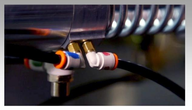
7. Once the cylinder is adjusted properly, tighten jam nut and reinstall the RED air line to cylinder
